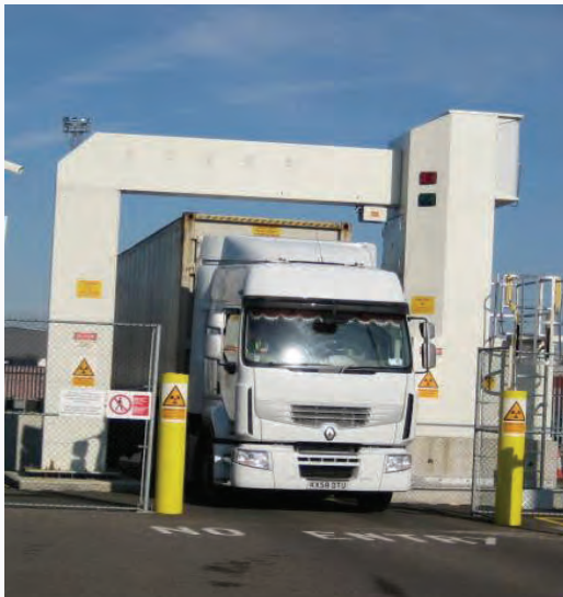
Mobile RPM equipment in Southampton 100% scanning pilot port in the United Kingdom (GAO)
