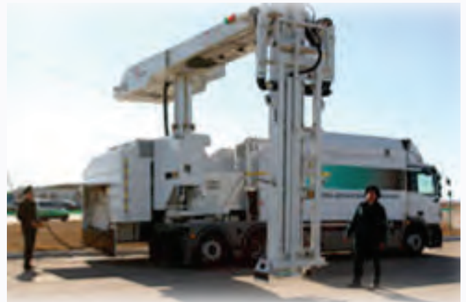
Mobile X Ray Unit, Copyright © Federal Customs Service of the Russian Federation
