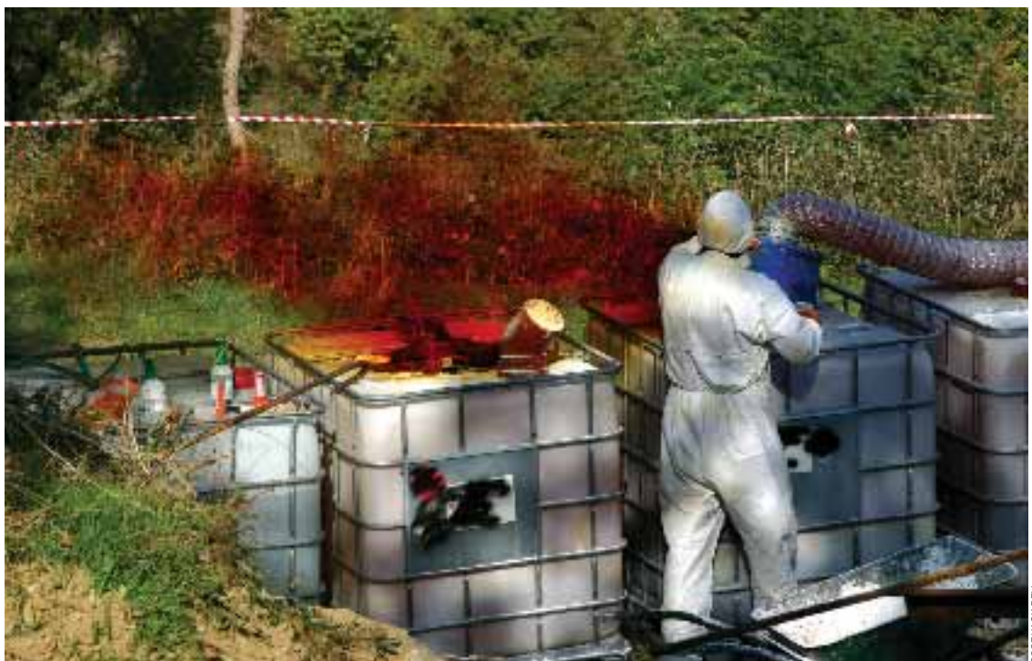
Transfer of Melange into intermediate bulk storage containers at a military storage depot in Albania in October, part of a project to dispose of the toxic rocket fuel
